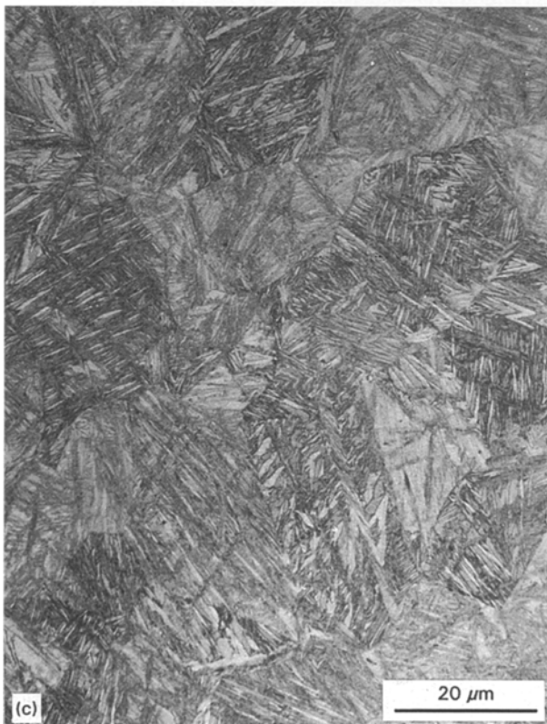
Figure 1 Microstructure observed after dipping in liquid nitrogen for 1 min: (a), (b), (c) and (d) represent optical images obtained from alloys 1, 2, 3 and 4, respectively.
